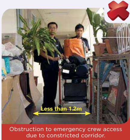
Ambulance crew and wheelchair-bound persons require at least a width clearance of 1.2m for access.
